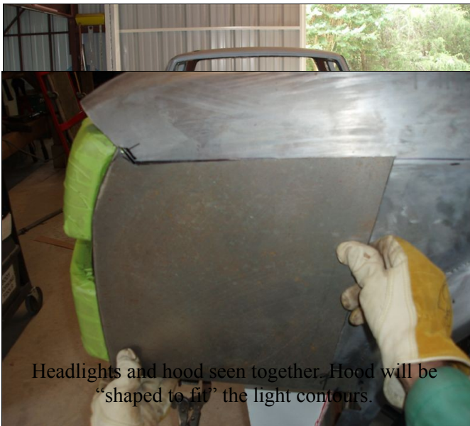
The hood is installed for testing and shaping the front area around the grill and lights
