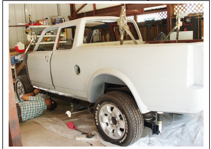
Adjustments being made while LT is almost completely set on frame.
