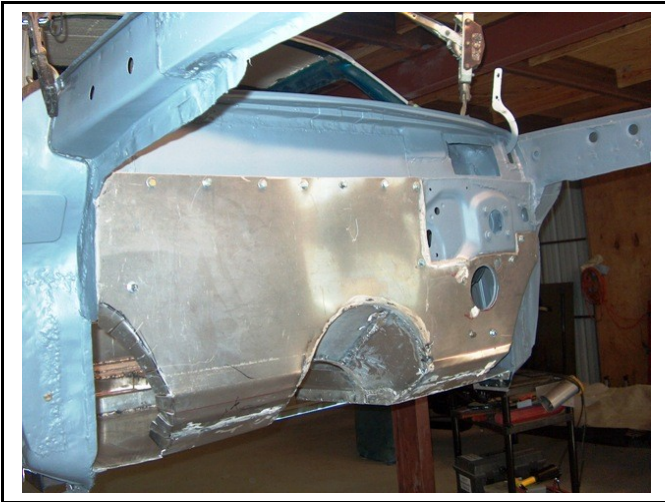
The firewall is fabricated of aluminum and filled in
