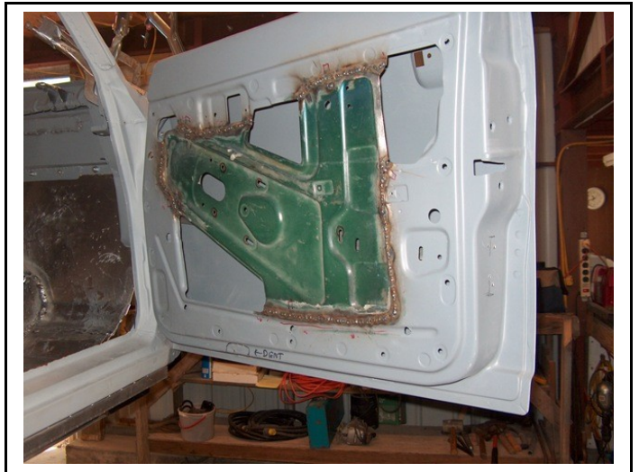
The P. side door panel section welded in place
